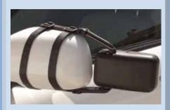
Prime's Clip On Tow Mirror easily installs with adjustable rubber straps to the O.E.M. mirror on most autos, vans, or pickups. It will not obstruct the vision of your existing mirror. No tools required for installation. Works great on the sport style mirror commonly found on Jeep Wagoneer, S10 pickups, and other hard to fit vehicles. Mirror arms extend approx. 7". To fit larger vehicle mirrors, use our "XL Clip On Mirror.
